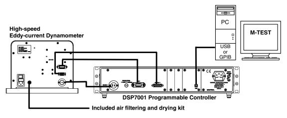
Figure 3–2 M-TEST-based configuration
