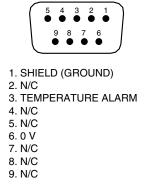
Figure 3–3 9 pin D-Sub temperature alarm connector
