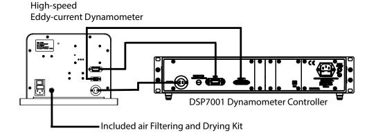
Figure 5–1 Calibration wiring
