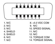
Figure 3–5 14 pin Centronic mini-connector
