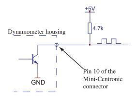
Figure 3–6 Example of a pull-up resistance supply
