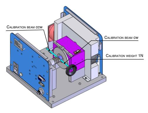
Figure 5–3 Calibration beams (CW side)
