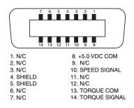
Figure 5–5 14 pin Centronic connector for torque signal measuring
