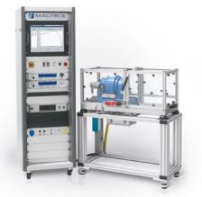
Fig. 3: Custom Motor Test System with WB brake
