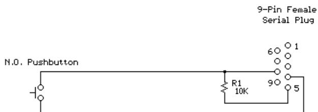
Use this diagram to construct a remote start switch for the Magtrol PF-TEST program. The N.O. switch may be either a momentary pushbutton to trigger a test, or a latching switch. A latching switch may be used along with a safety cover over the motor to control the test. You must specify the type of switch used in the Hardware Configuration of PF-TEST. The switch will function only in the COM2 port of the computer.
