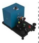
The Micro Dyne dynamometer absorbs power with Magtrol's unique Hysteresis Braking System. Because it does not require speed to create torque, the dynamometer can conduct a full motor ramp—from free-run to locked rotor.
