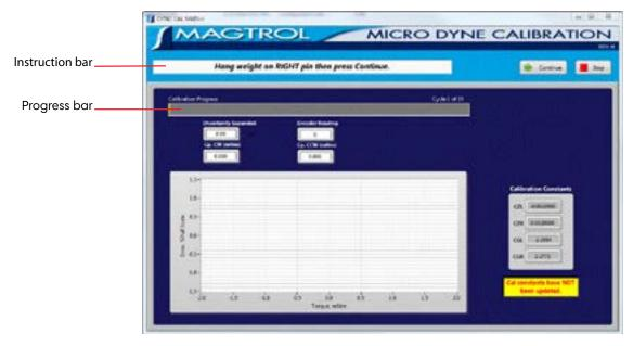
Fig.6-4 Calibration Instruction and Progress Bars
