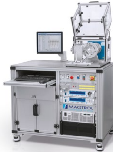
Fig. 5: Custom Motor Test Bench for Automotive Industry
