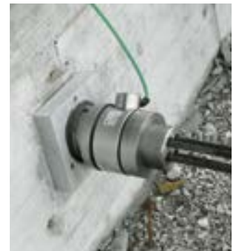
Fig. 2: HRL-4-1000 (4 strands) mounted on cable anchor
