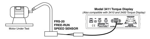
NOTE: The FRS-20 can also be used with the DSP7000. The FRS-22 can be used with the DSP7010. The 3411/DSP also supplies power to the FRS Sensor.
