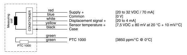
Fig. 2–12 DI 63X displacement transducer connecting cable
