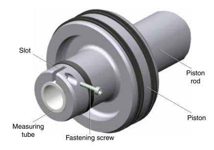
Fig. 2–9 Measuring tube fixing by clamping
