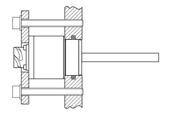
Fig. 2–7 DI 510/111 displacement transducer mounting
