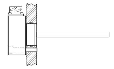
Fig. 2–5 DI 510/011 displacement transducer mounting
