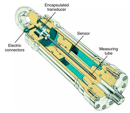
Fig. 2–2 Installation of both transducer parts
