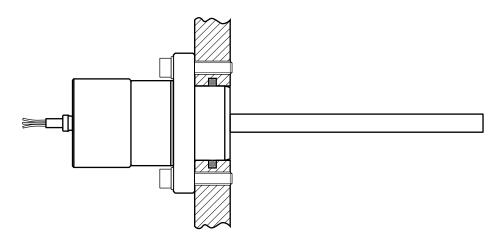
Fig. 2–6 DI 630/021 displacement transducer mounting
