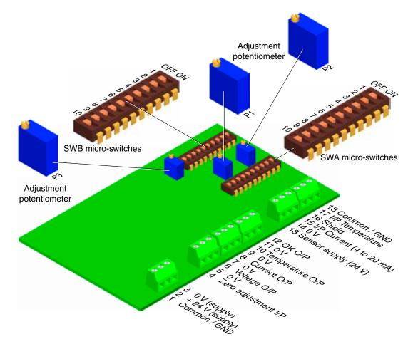
Fig. 4–1 Position of the adjustable components on the board and terminal allocation
