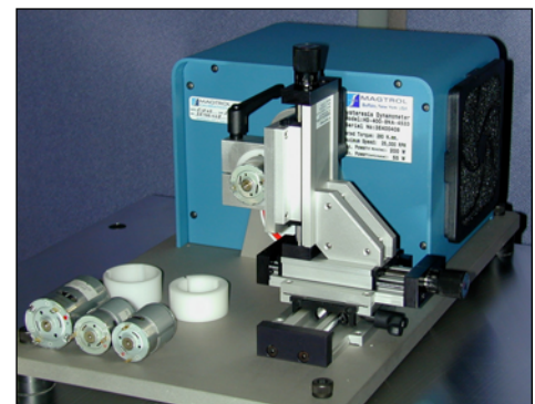
Custom motor fixture with sliding platform.
