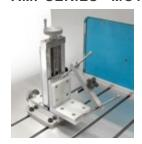
Magtrol's AMF Series Adjustable Motor Fixtures are used to secure small to medium-sized motors in place while running any test. These extremely versatile fixtures also enable easy motor centering for coupling to a brake.
