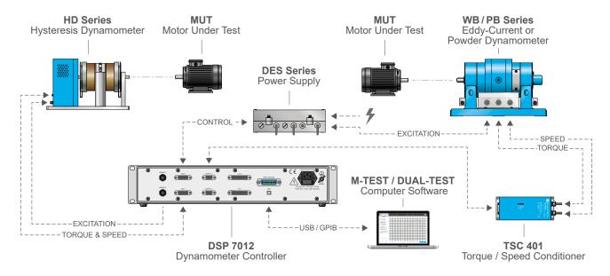
This configuration allows two systems to be controlled by the same DSP7012. It can be either a test bench for testing two motors of different types (or the same motor with two different characterizations).
