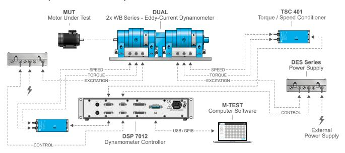
DUAL System allows you to take advantage of two complementary WB Series Eddy-Current Dynamometer. The unique DUAL Dynamometer System increases torque while maintaining high rotational speed.
