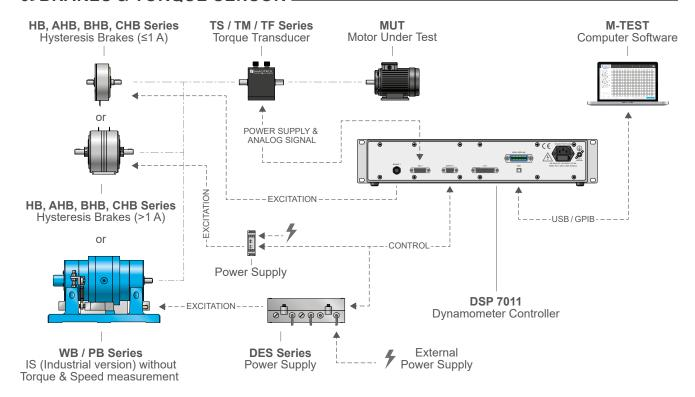
Alternative for standard configuration #1 or #2. The single-channel DSP7011 controls a Hysteresis Brake or Dynamometer and acquires the signal from an external Torque Sensor. The DSP7011 also serves as an interface for PC connection (M-TEST software). The advantage of this configuration lies in the scalability and modularity of the components.
