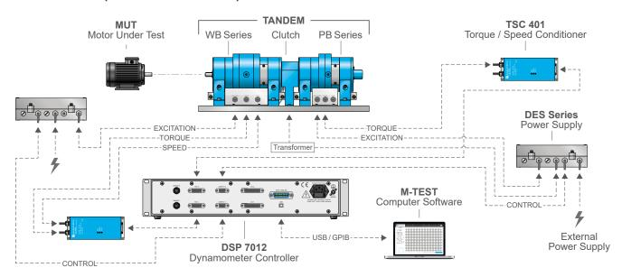
TANDEM System are composed of 2 Dynamometers; one WB Series Eddy-Current Dynamometer and one PB Series Magnetic Powder Dynamometer, connected by an automatically disengageable clutch.
