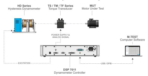
In a similar way, but differently from configuration #1, torque is measured using an external torque transducer, rather than the one integrated in the HD Series Dynamometer. The advantage of this extended configuration lies in the measurement accuracy of the torque transducer, which is more accurate than the one integrated in the dynamometer.
