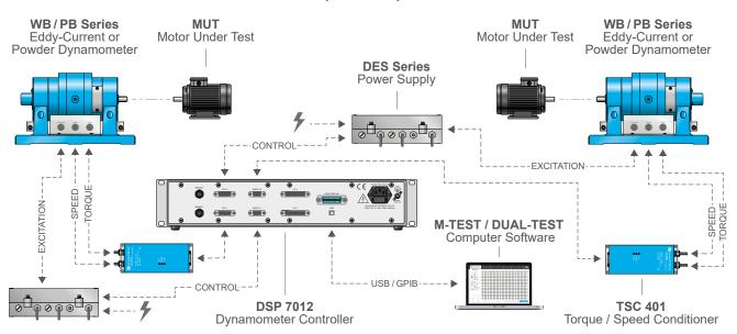
Similar to configuration #7, this configuration allows testing with two WB Series (Eddy-Current) or PB Series (Magnetic Powder) Dynamometers with different characteristics. A dual-channel DSP 7012 is required to drive all the accessories required (TSC, DES Series).
