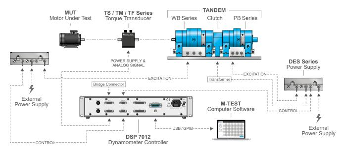
Similar to configuration #9, this configuration allows testing with TANDEM system (two Dynamometers), while benefiting from increased precision thanks to the torque transducer.
