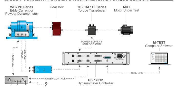
Alternative to configuration #5 using a WB Series (Eddy-Current) or PB Series (Magnetic Powder) Dynamometer. In this configuration, a dual-channel DSP 7012 is required to instrument all components.
