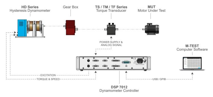
This configuration combines modularity and precision. Thanks to the various components, it is possible to measure the efficiency and effectiveness of the motor and gearbox individually, but in a single test system.
