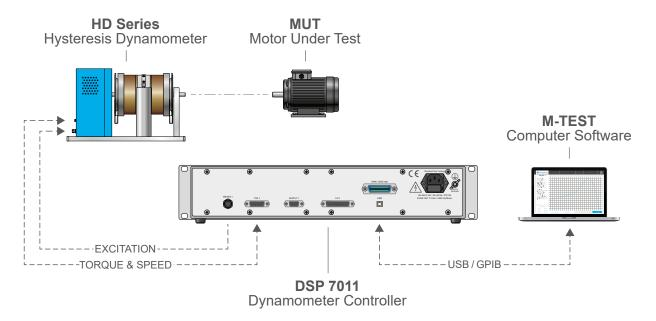
Easy-to-use standard configuration. The HD Series Dynamometer provides both braking power and torque measurement.
