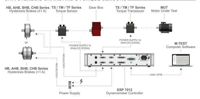
Alternative to configuration #4. A dual-channel DSP 7012 is required to instrument all components. Differently from configuration #4, the performance measurement and efficiency of the motor and gearbox can be calculated with greater precision.
