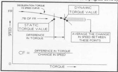
increasing torque load, and fetch a group of test points. We have selected the first data point where the speed will be just less than 78% of the Free Run speed. Call this the dynamic speed value. Additionally, save one test point before this value, and one after. Immediately program the 4629B (Nddddd) to a speed exactly equal to this "dynamic" value. When the speed has stabilized, fetch this as the static torque value.
