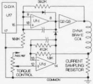
The front panel TORQUE control adjusts a voltage input to a differential operational amplifier - U1d. This voltage is compared against a voltage analogous to the brake current. The difference is amplified and applied to the Dynamometer Brake.
