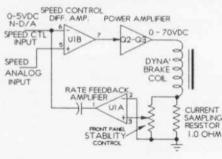
U15, pin 15 of SCC-1, this signal is applied to the *inverting* input of differential operational amplifier - U1b. The *non-inverting* input is the reference input "N-D/A," established by the main processor from external instructions. The difference, amplified, commands the torque level of the Dynamometer Hysteresis
