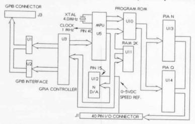
the 4629B operating system. There is a 2K non volatile RAM device identified as U11. The N-D/A speed reference D/A is U12. U13 and U14 are Peripheral Interface Adapters. U1, U2, and U3 are the GPIB interface control elements. The balance of the components are buffer and timing control devices.
