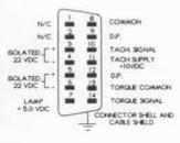
Pin 10 is the tachometer frequency signal providing 60 pulses per shaft revolution. The signal level has a low voltage of .2  $\pm$ .1 and a signal high of 1.0  $\pm$ .2 VDC. The common to this signal is Pin 8.
