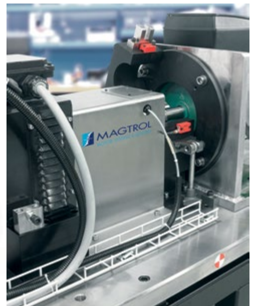
Fig.2-6 Test bench with fixed and movable metal guard with safety switch.
