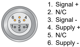
Fig.5-10 Connector Pin Configuration for WB/PB 43 Dynamometer Torque Signals
