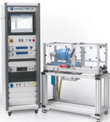
Fig. 6: Custom Motor Test System with WB brake
