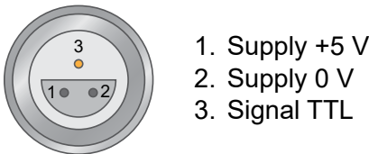
Fig.5-12 Connector Pin Configuration for WB/PB 43 Dynamometer Speed Signals
