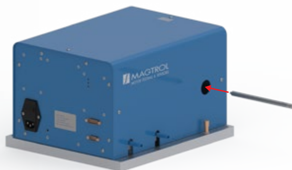
Fig.7-3 Mount the calibration arms
