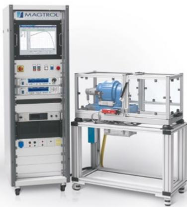
Fig.3: Custom Motor Test System with WB brake
