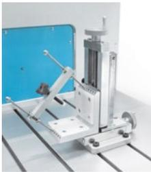
Magtrol's AMF Series Adjustable Motor Fixtures are used to secure small to medium-sized motors in place while running any test. These extremely versatile fixtures also enable easy motor centering for testing. These accommodate motors up to 101 mm (4") in diameter.
