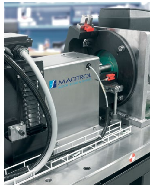
Fig.2-12 Test bench with fixed and movable metal guard with safety switch.
