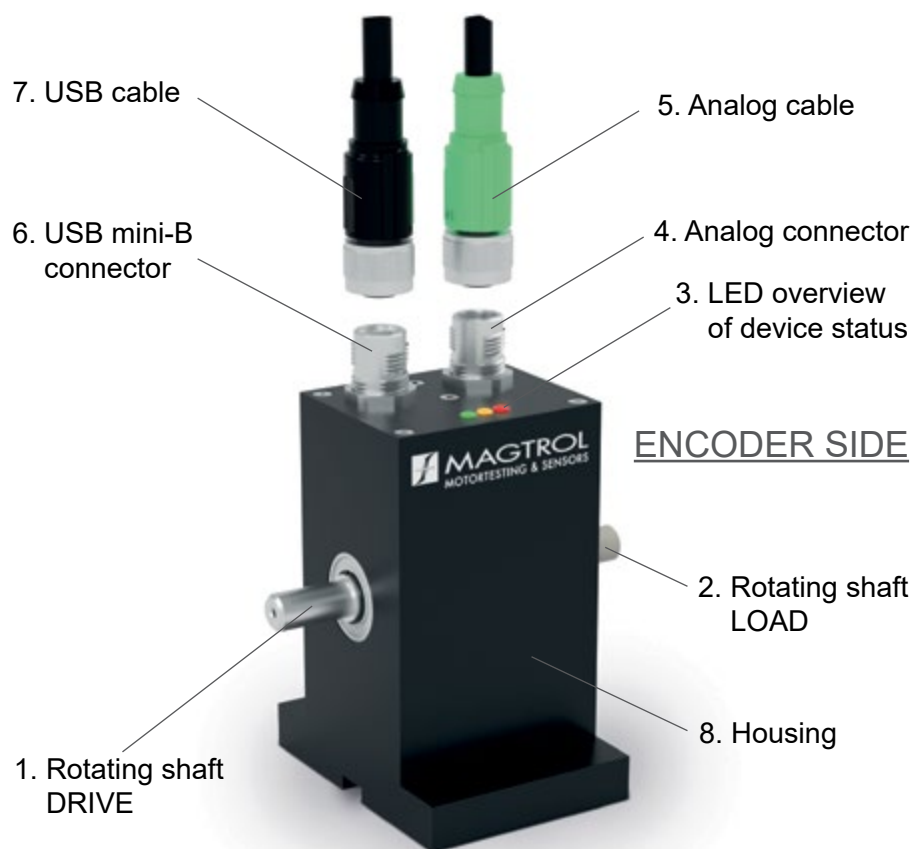
Fig.1-2 Description of the TS Series torque transducer parts
