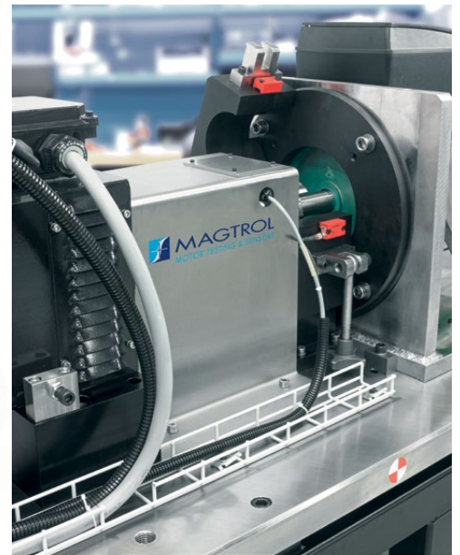
Fig.2-24 Test bench with fixed and movable metal guard with safety switch.
