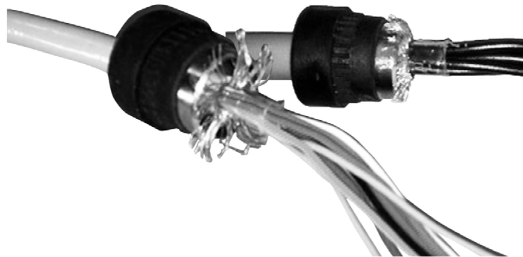
Fig.2-8 Connect Shield of EMC Stuffing gland
