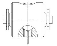
Figure 1-1 Mercury Cell
