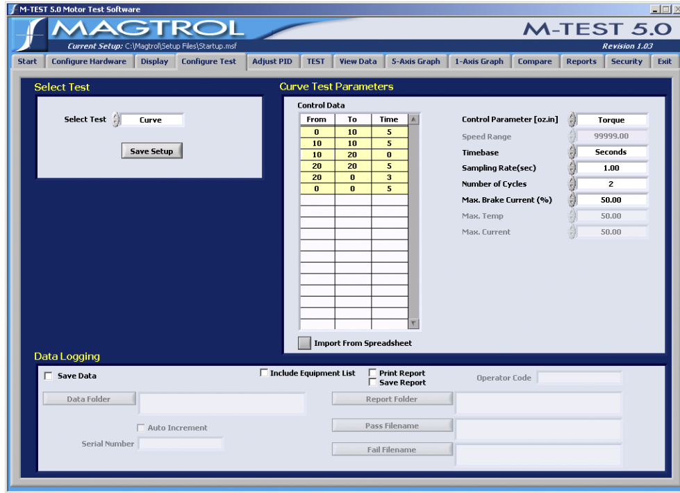
Figure 7-6 Torque Curve Setup Example
