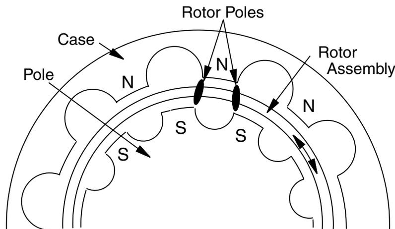
Fig.3-2 Hysteresis Brake Cross Section
