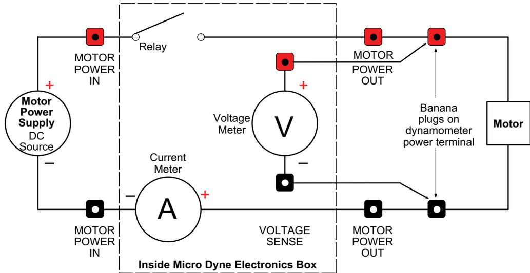
Fig.2-4 Basic Motor Power Circuit
