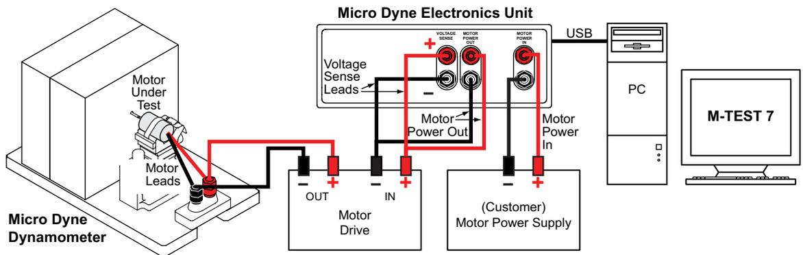
Fig.2-7 Motor Drive Configuration
