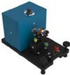
The Micro Dyne dynamometer absorbs power with Magtrol's unique Hysteresis Braking System. Because it does not require speed to create torque, the dynamometer can conduct a full motor ramp—from free-run to locked rotor.
