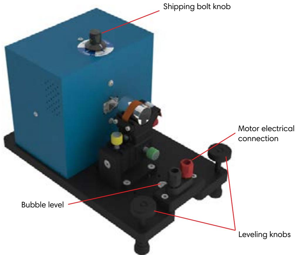
Fig.2-1 Micro Dyne Dynamometer
