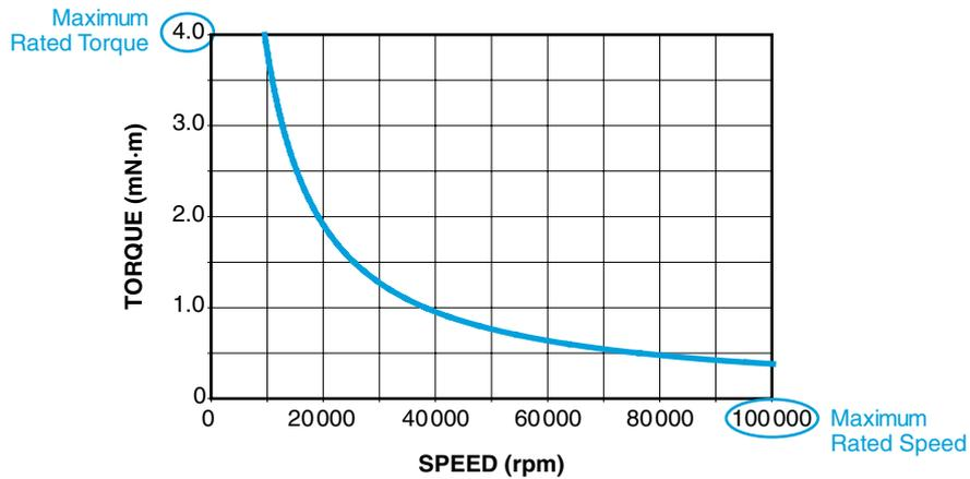
Fig.3-1 Micro Dyne Power Absorption Curve
