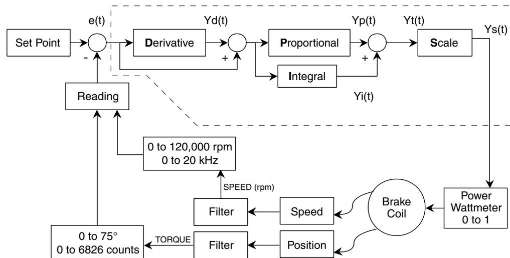
Fig.5-3 Control Loop and PID System Block Diagram
