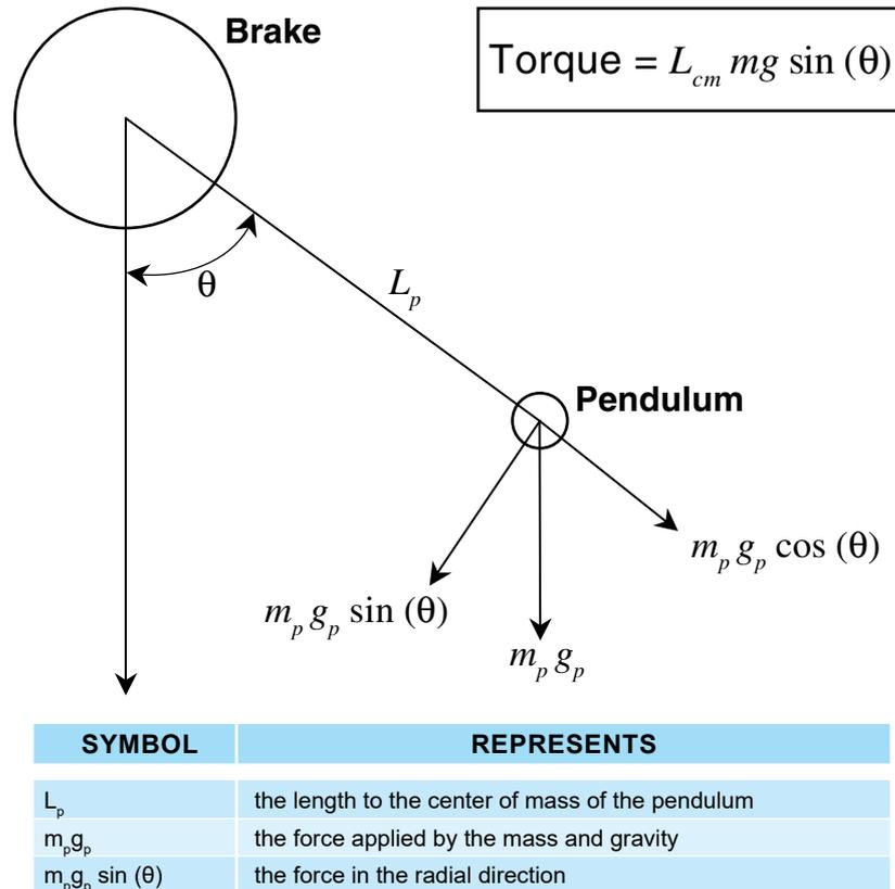
Fig.5-1 Illustrated Torque Principle
