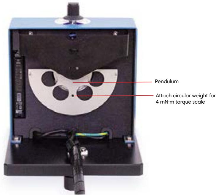
Fig.4-1 Dynamometer, Inside View
