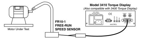
NOTE: The FR10 Free-Run Sensor can also be used with Magtrol's DSP6001 Dynamometer Controller.
