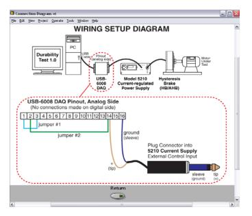
Figure 4-4 Wiring Setup Diagram
