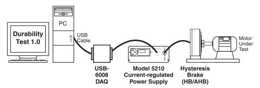
Figure 1–1 Durability Test 1.0 System Configuration
