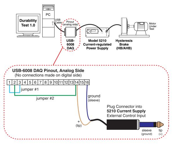
*Figure 2–1 USB-6008 Wiring Diagram*
