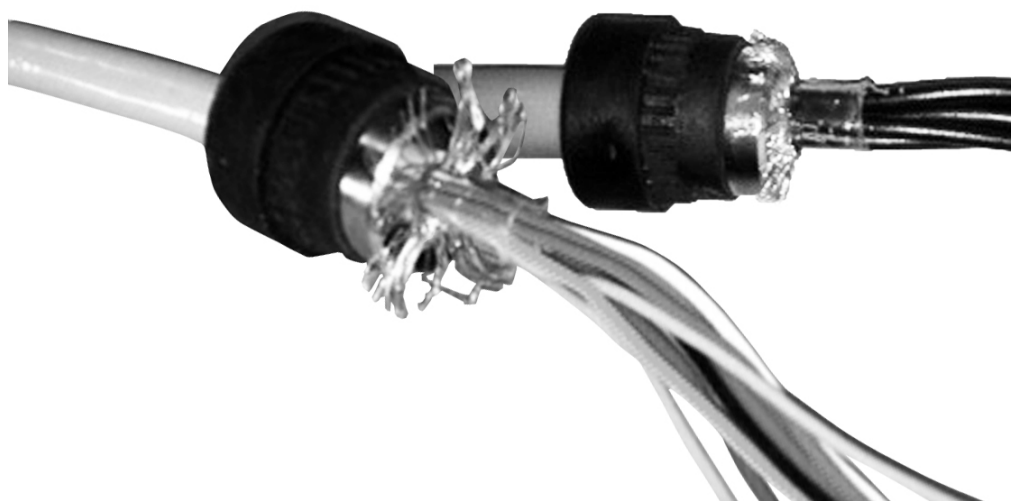
Fig.2-8 Connect Shield of EMC Stuffing gland
