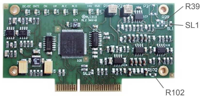
Fig.2-13 Location of resistors & solder links on the DES Series circuit
