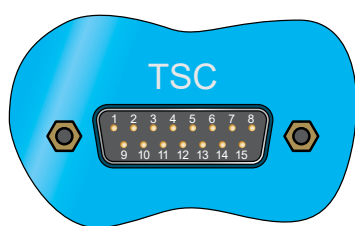
Fig.5-9 Connection socket for the torque and speed signal.
