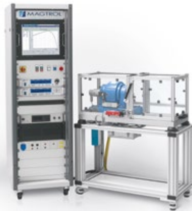
Fig. 3: Custom Motor Test System with WB brake
