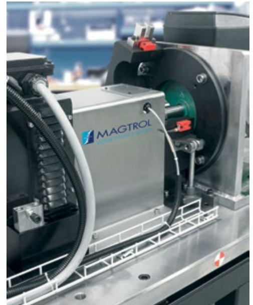
Fig.2-5 Test bench with fixed and movable metal guard with safety switch.
