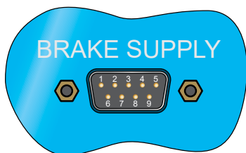
Fig.5-11 Connection socket for the dynamometer brake supply
