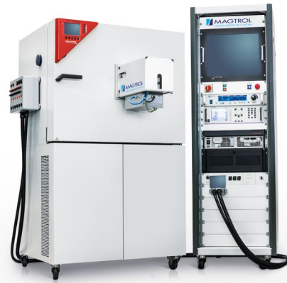
System for certification of automotive electric motors in specific climatic conditions.
