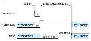
The stator will turn *ON* power to the rotor. The first 5.5s of information will be used for rotor voltage measurement. Note during this time, the «analog output» and USB are set to zero.
