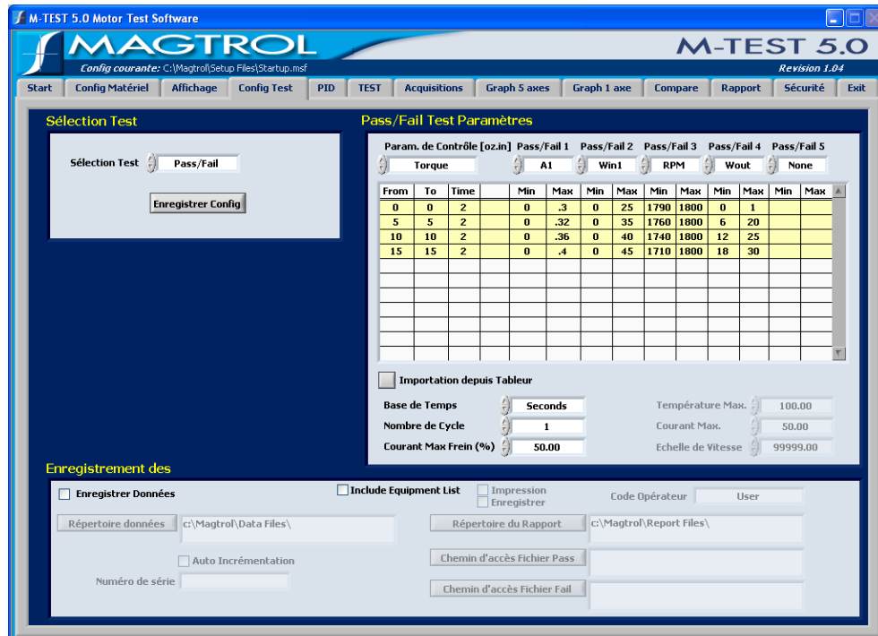
Figure 7-8 Configuration d'un test Pass/Fail
