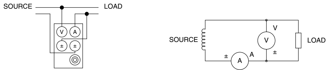
Figure 3-7 Single-Phase, Two-Wire Wiring Schematic
